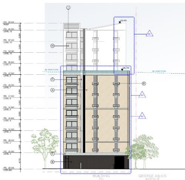
Figure 38: Northern elevation of Building D1, showing the height non-compliance in blue
